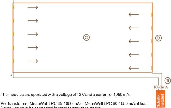
Per transformer MeanWell LPC 35-1050 mA or MeanWell LPC 60-1050 mA at least 3 modules must be connected in order to prevent burnout.
